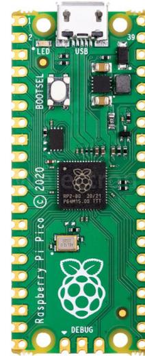
RP2040 is a low-cost, **high-performance microcontroller** device with **flexible** digital interfaces.
